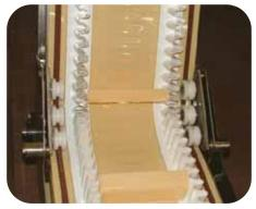
SuperDrive™ Z-elevator with Flights, Guides and Sidewalls
