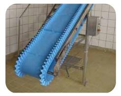
SuperDrive<sup>™</sup> with Sidewalls and Special Flights
